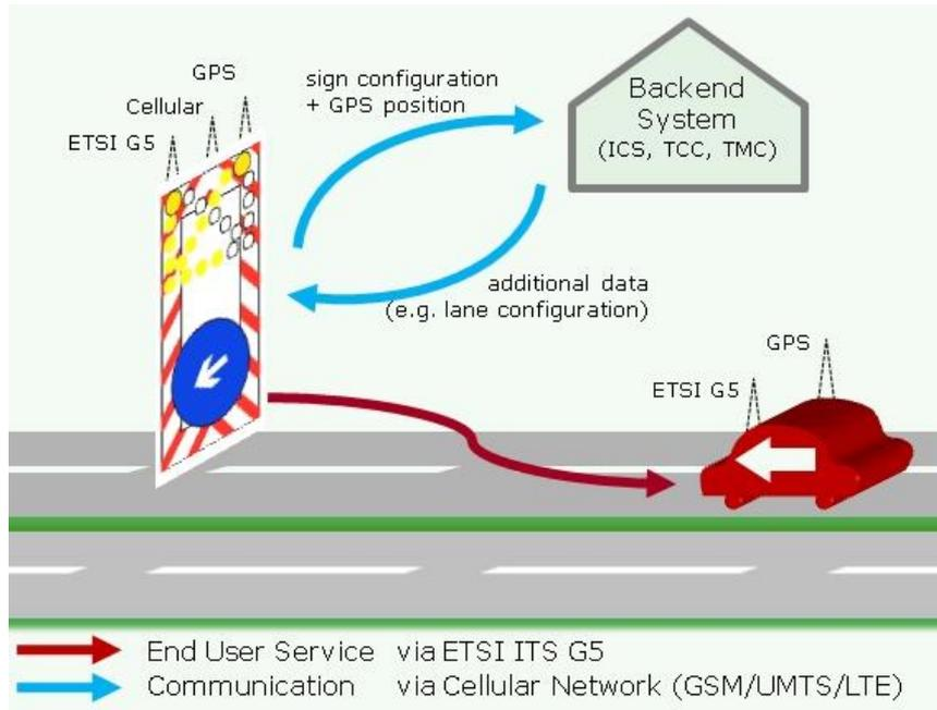
Figure 2 Use case illustration for Road Works Warning in “Basic Service” mode
