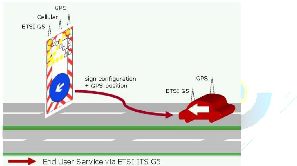
Figure 1 Use case illustration for Road Works Warning in “Stand-alone” mode
