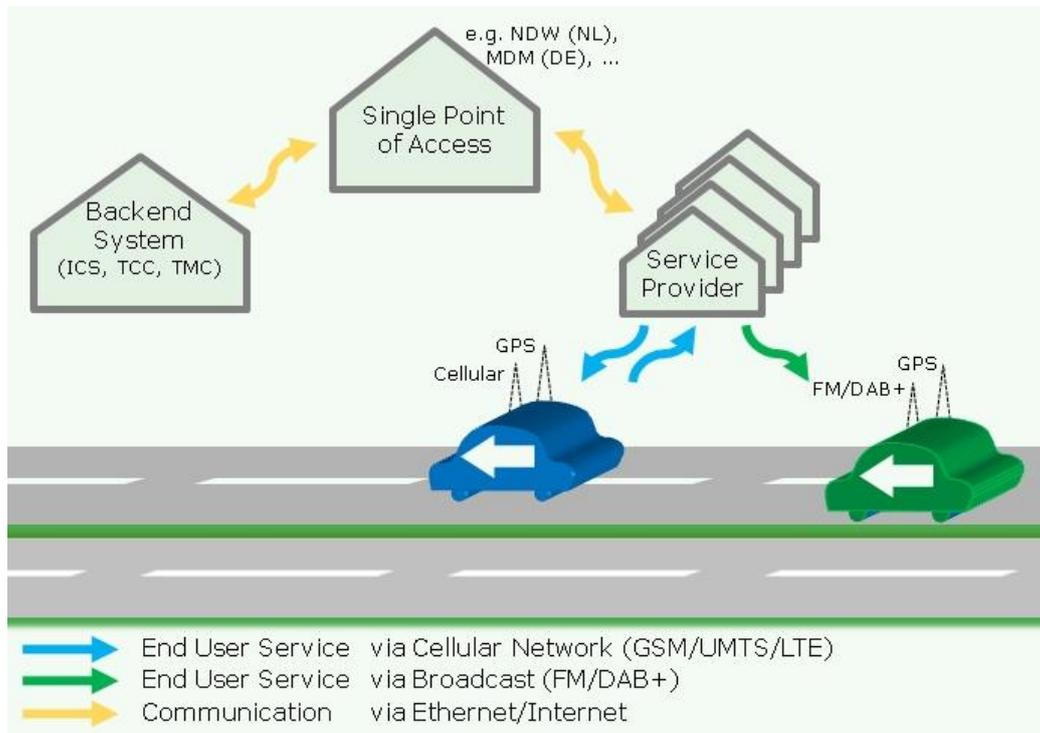
Figure 4 Use case illustration for distribution of Road Works Warnings via Service Providers
